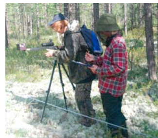
Figure 17. Buckner point-intercept sampling device. The box on the end piece of the device contains a mirror that can be pointed down to the ground cover or up to the forest canopy. The tube is a telescope that magnifies the image in the mirror. Cross hairs in the sighting device identify a point that intercepts a plant species which is recorded as a “hit”. The percentage cover of an individual species or cover type is the number of hits for that type divided by the total number of hits. Photo no. DSC_0151, 8/06/07, D.A. Walker.
