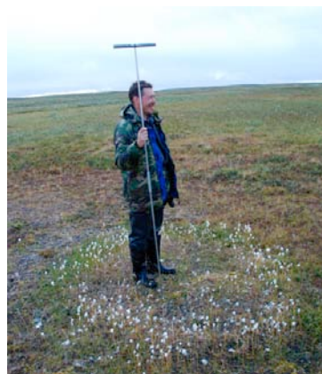
Figure 19. Anatoly Gubarkov with active-layer probe used for measuring depth to the permafrost table. Photo no. DSC_0180, 8/27/07, D.A. Walker.
