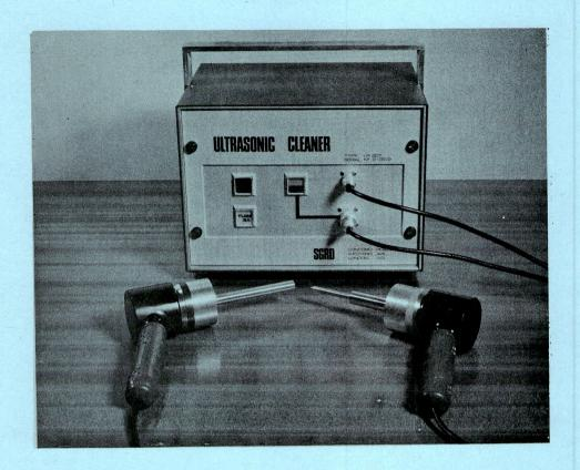
The SGRD Limited ultrasonic pistol cleaner, as used in museums world-wide, can considerably reduce the time required for preparing rock covered fossil bones for exhibition. For example, it has been calculated that some two years work could have been needed to clean 200 specimens by conventional methods. By using the ultrasonic instrument the cleaning time amounted to 15 months.
