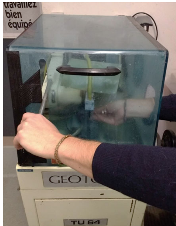
Fig. A.9 Precision slicer to reduce the specimen thickness to 1 mm
