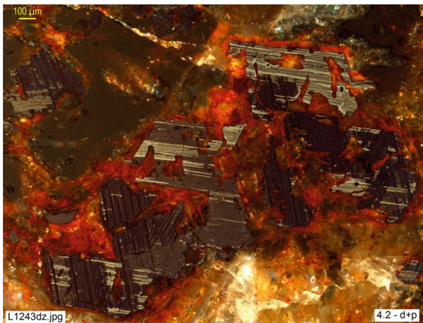
Fig. 1.2 Same image observed with the analyzer ( d + p ): the internal lamellar-octahedral structure (known as Widmanstätten's ) is revealed by the appearance of thin lamellae of ilmenite and martite arranged as planes (111) of titanomagnetite
