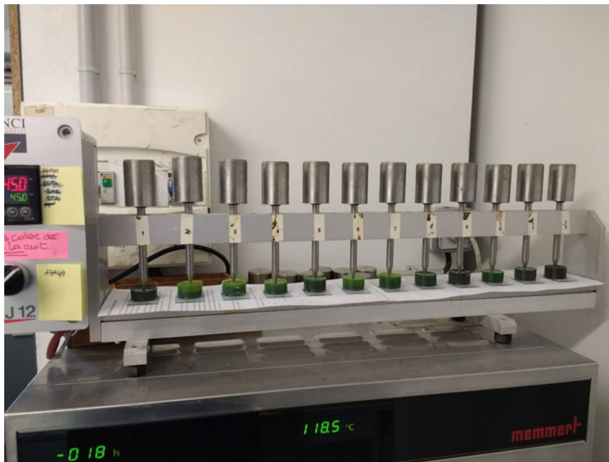
Fig. A.8 Drying test specimens glued to slides
