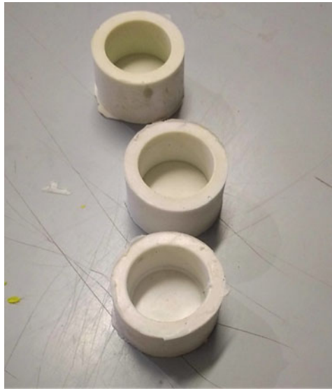
Fig. A.3 Cylindrical silicon molds. This format allows the same sample to be studied both in the AMCO system and in an electron microscopy system or by traditional methods
