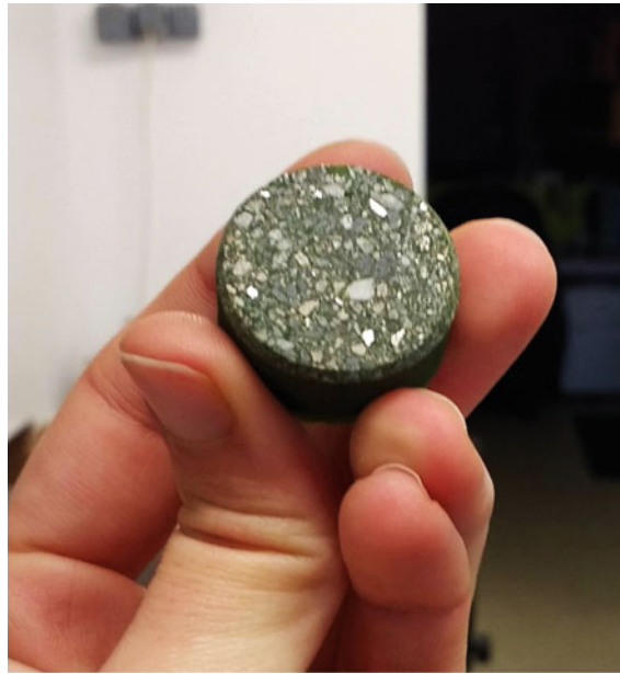
Fig. A.6 Preparation of the specimen surface to be glued to the object holder glass. A light roughening is done to even the surface, and to facilitate gluing the edges are rounded with the same polishing machine
