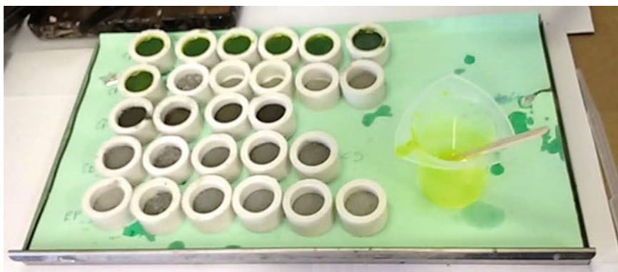
Fig. A.5 Embedding of ground samples in fluorescent resin
