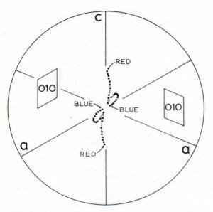
Fig. 6. Position of the optic axes in monochromatic light. Stereographic projection. Red:  $\lambda = 670 \ m\mu$ . Blue:  $\lambda = 470 \ m\mu$ .
