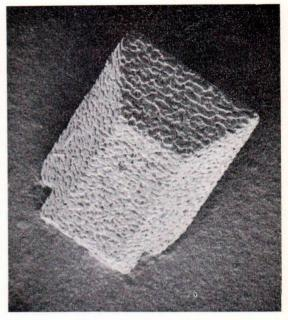
Fig. 1. Crystal habit of sub-calcium olivine. Scanning electron micrograph, 850 ×.
