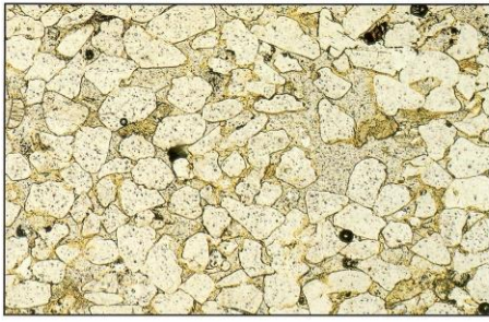
109 Quartz Arenite in plane-polarized light. Locality: New Red Sandstone, Permo-Trias, England (x 47).
