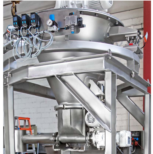
FEEDOS M integrated in the DIW-3E frame scale for high accuracy gravimetric feeding
