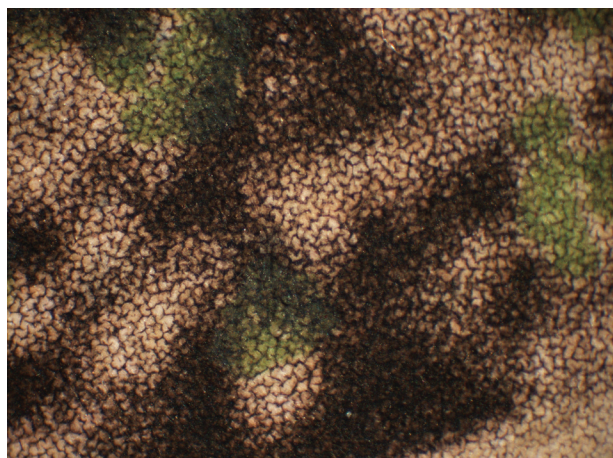
Figure 18a Black ink area of the color collotype in fig. 17 at 40× magnification.
