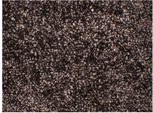
Figure 6f Microscopic structure of the Dmid area of the collotype print in fig. 5 at 40x.
