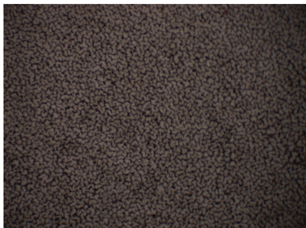
Figure 6c Microscopic structure of the Dmin area of the collotype print in fig. 5 at 40×.
