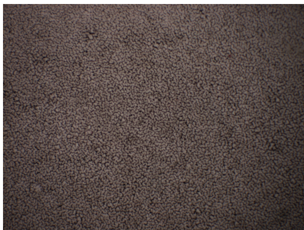
Figure 6b Microscopic structure of the Dmin area of the collotype print in fig. 5 at 25×.
