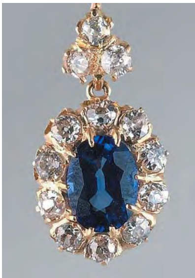
Figure 15. The 8.00 \times 6.20 \times 3.80 mm blue stone in the center of this yellow-metal cluster earring set with “old cut” diamonds proved to be a bulk-diffused synthetic sapphire.
