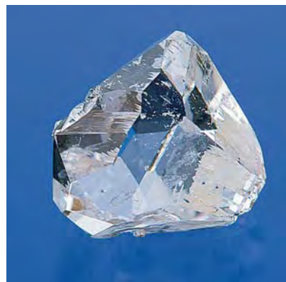
Figure 2. This 5.84 ct synthetic BeO crystal was grown experimentally in Russia.
