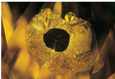
Figure 9. The tension halo in this 1.20 ct orange-yellow diamond appears similar to the one in figure 8. In this case, however, the sugary texture and undulating nature of the halo suggests that this diamond has been exposed to an HPHT process, which was confirmed by spectroscopic analysis. Magnified 45 \times .
