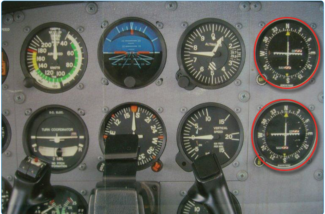
Figure 2-52. Instrument panel with dual VORs.
