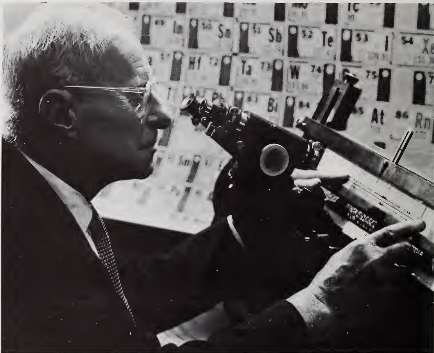
W. F. Meggers prepares to measure one of the spectrograms on which these tables of spectral-line intensities are based.
