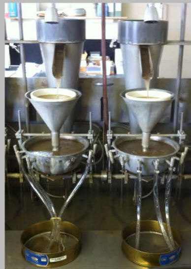
Samples are run through an elutriator to separate roots and J2s.
