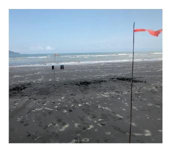
Sampling stations were marked with flagged bamboo wands between the high tide zone and shallow subtidal.
