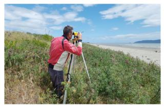
Cross-shore profiles from the top of the dunes to the shallow subtidal were measured using a theodolite.
