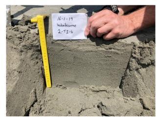
Box corer hole showing clean sands with no enrichment visible.
