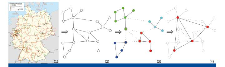
Fig. 16: Schematic diagram of developed linear solver: Physical grid (1) is represented as undirected graph (2), graph after partitioning (3), coarse grid correction (4).
