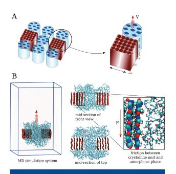
Fig. 21: Friction between crystal and amorphous phase. (A) Scheme of crystals (brown) embedded into amorphous matrix bundles (blue). (B) Lateral sliding of the two phases allowed for determining the inter-phase friction.
