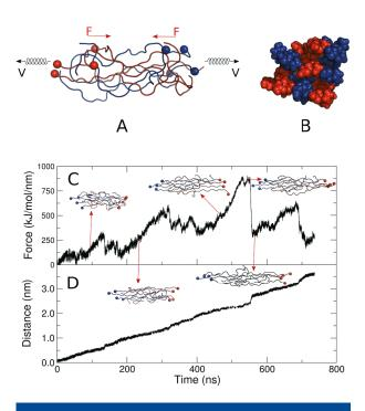
Fig. 20: Silk is a viscoelastic material, and the viscosity can be mainly attributed to its amorphous phase. (A,B) A representative fraction of the amorphous phase was pulled in MD simulation. (C,D) Forces encountered during pulling allowed for determining the internal molecular friction in silk fibers.
