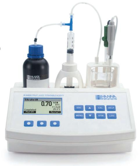
The HI84532 incorporates a precise piston dosing system, which allows for a highly accurate determination of the amount of titrant used. It is capable of dynamic dosing, making testing both faster and more accurate. Pump calibrations, performed with the provided Hanna standards, help assure the measurement accuracy.
