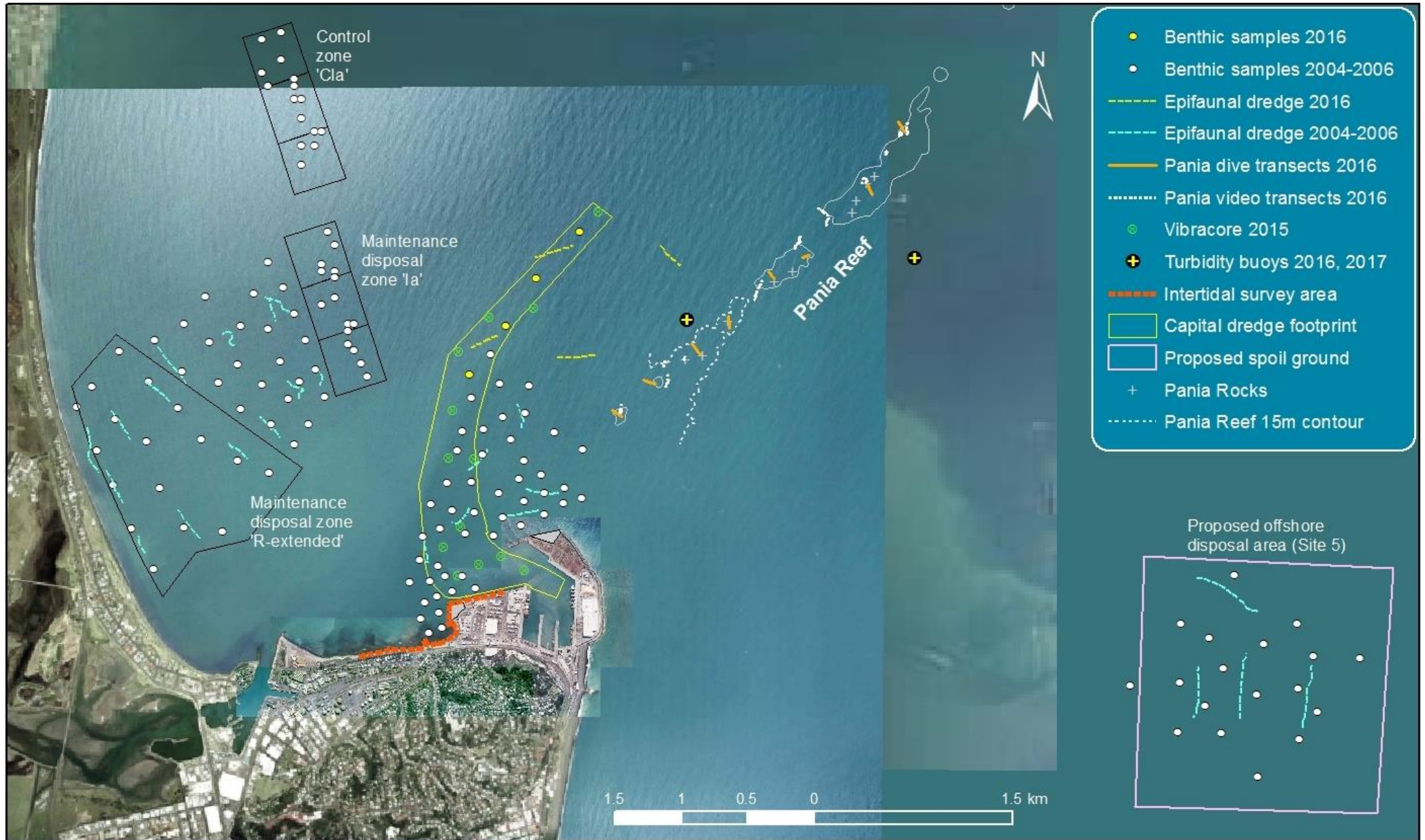
Figure 2. Overview spatial layout of benthic survey components for the Port of Napier, Westshore Beach, Pania Reef to offshore Marine Parade.
