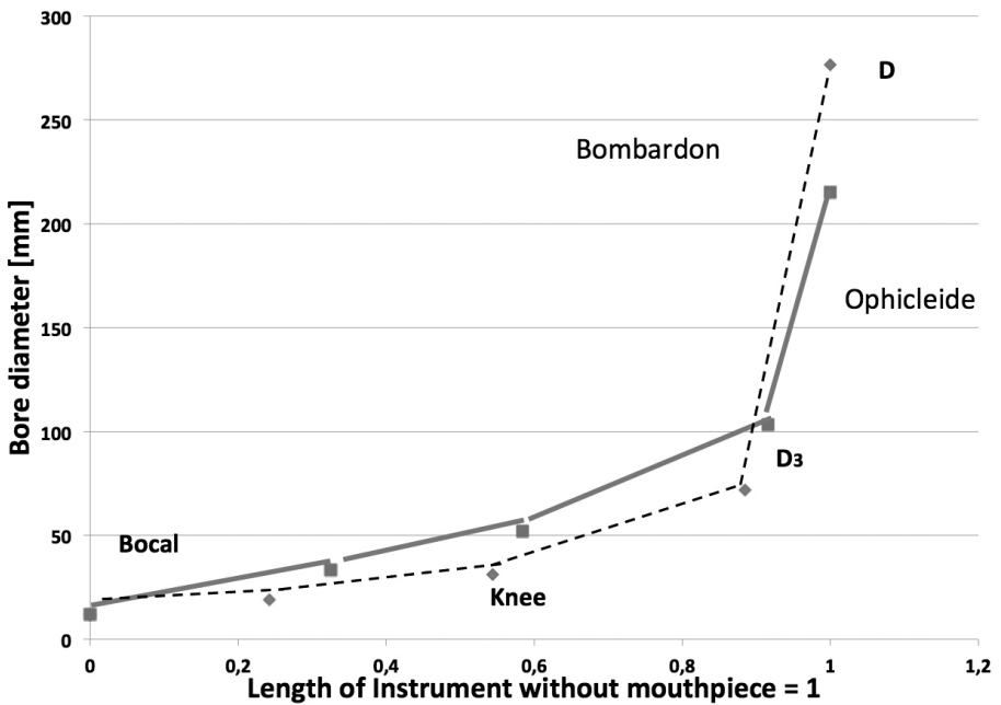
Figure 22: Bore diameters: bombardons in ophicleide-shaped in C (average of 3 instruments) and French-style ophicleides in C and B \flat (average of 14 instruments).
