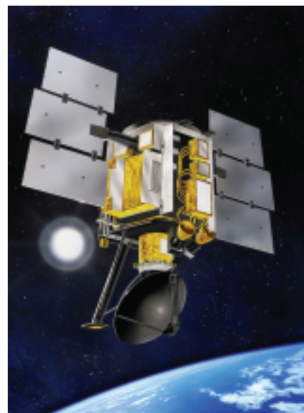
Figure 1: An artist's rendition of the QuikSCAT satellite, which was launched in June 1999. The dish-like object at the bottom is the SeaWinds Scatterometer.
