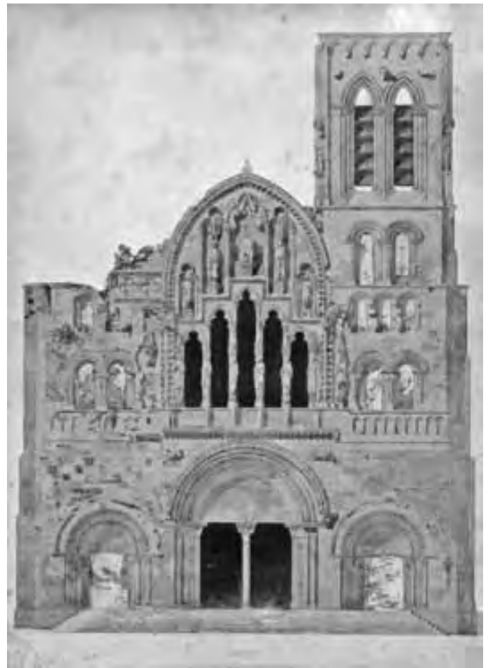
Figure 187. The Madeleine, Vézelay, the west elevation. Measured drawing before restoration by E. Viollet-le-Duc,
