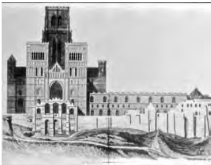
Figure 151. John Carter: Durham Cathedral, west elevation with reconstructed finishing of the west towers
