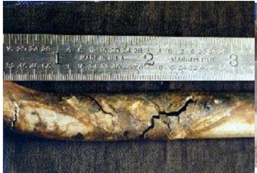
Brittle fracture Problem induced Corrosion Stress Oxidation Cracking
