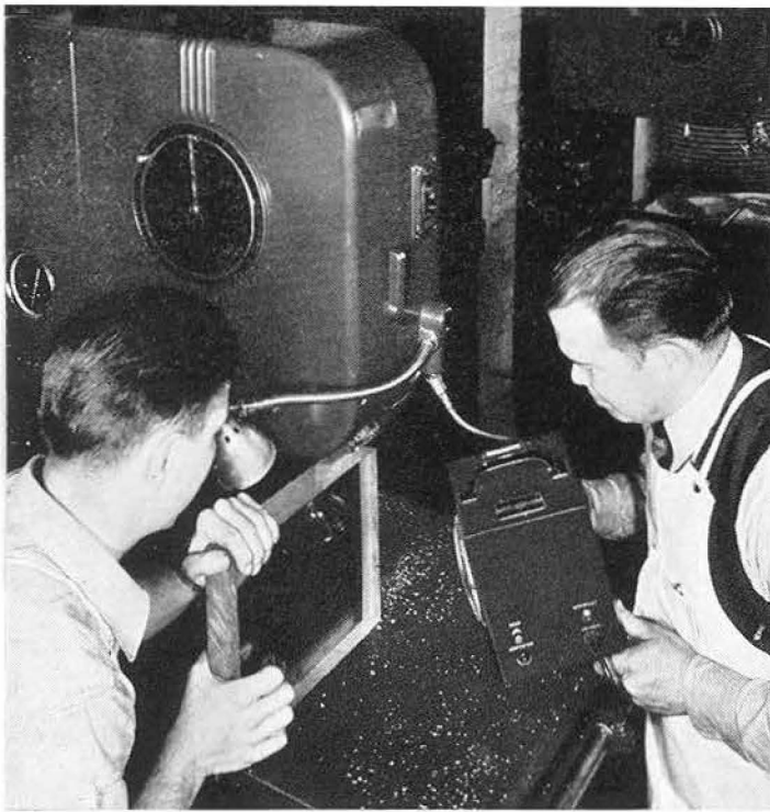
FIGURE 5: Photograph courtesy Continental Machines, Inc. Continental Machines and its associated DoAll Company use the Strobotac in the design of band saws, contour saws, and band filing machines. This photograph shows the Strobotac used in watching the action of a DoAll band saw cutting a slab of transparent plastic to see the cutting action of the saw teeth and to isolate and to analyze vibration.
