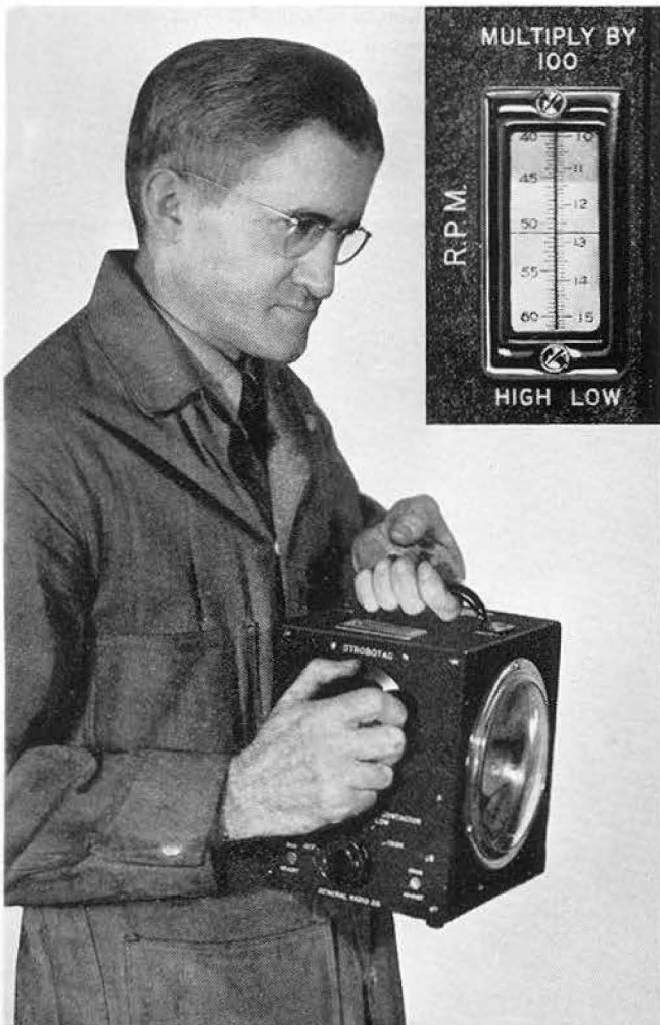
FIGURE 4: When the Strobotac is held in operating position, the speed scale (shown in inset) is at the top where it can be easily seen by the operator.
