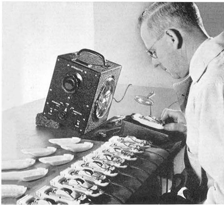
FIGURE 7: Photograph courtesy Remington-Rand, Inc. An application of the Strobotac in modern production testing. Adjusting the cutters of electric shavers for optimum operation.
