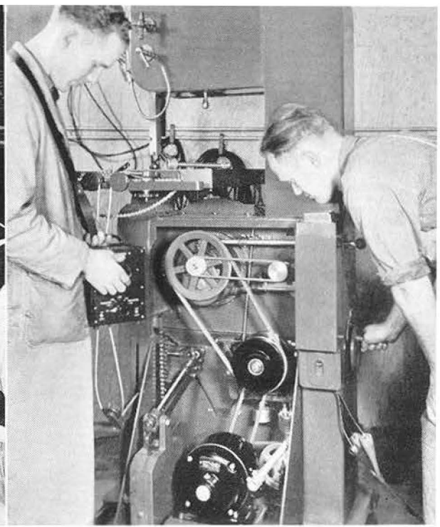
FIGURE 6: Photograph courtesy Continental Machines, Inc. All DoAll machines are equipped with a Speedmaster Variable Speed Pulley. The Strobotac is used to study the mechanics of the Speedmaster, particularly the effect of various torques in order to detect and to correct excessive slippage and vibration.
