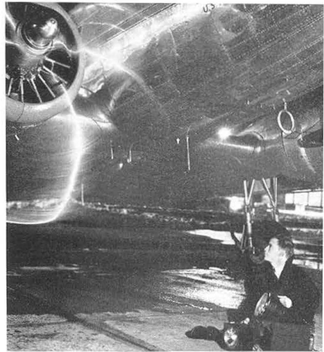
FIGURE 9 (above): Photograph courtesy American Airlines. The Strobotac and Strobolux aid the design of propeller counterweights by showing the performance at high speeds by means of the slow-motion effect.
