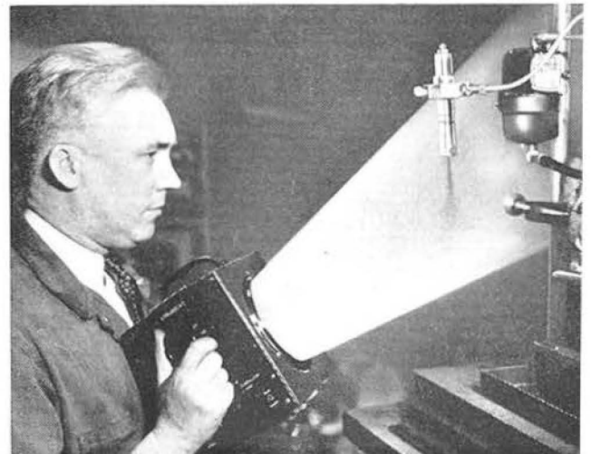
FIGURE 10 (above): Photograph courtesy Cleveland Wire Spring Company. Valve spring operation is studied in slow motion with the Strobotac.
