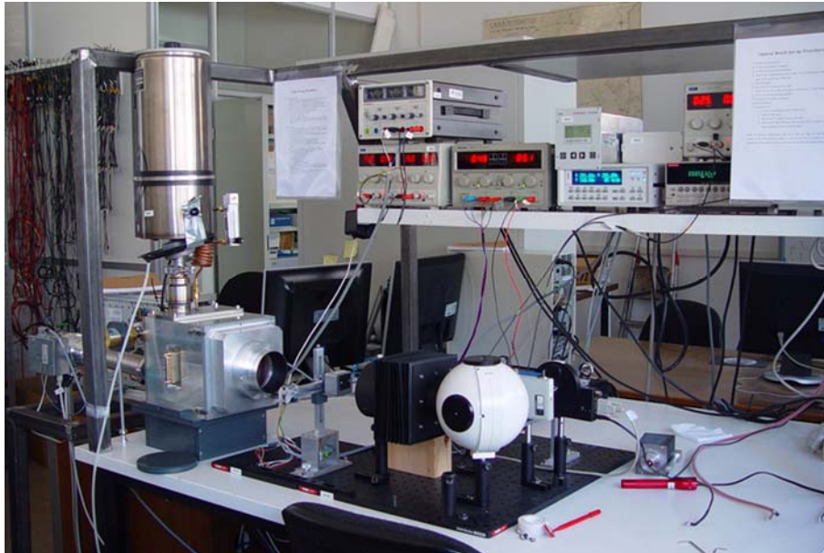
A photograph of the test bench to test the DES electronics. To the left of the picture one can see the cube that contains the CCD together with a small liquid nitrogen Dewar, to maintain it cold. On the right there is an optical system to illuminate the CCDs. The electronics are inserted in a crate in the back of the picture (not seen).
