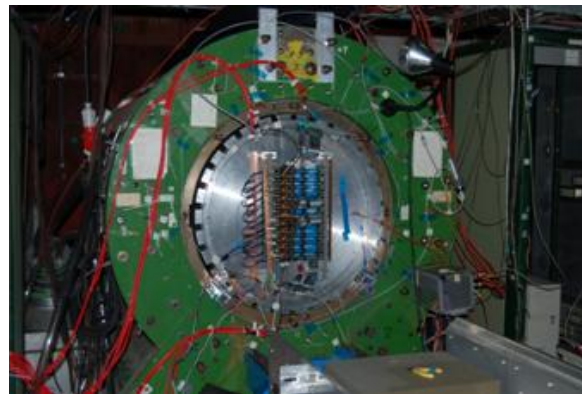
The readout prototype inside the magnet (green) and the HARP field cage (aluminum).
