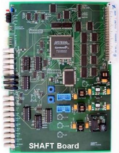
Top layer of the 6-layers SHAFT board, designed and built at IFAE (left); example of monitoring of the stability of the PMTs of one of Tilecal module.
