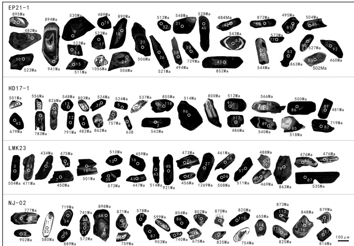
Fig. 4. Zircon CL images and LA-ICP-MS spot locations. The circles and numbers in the Zircons are the locations and analysis numbers of the laser ablation spot, and the numbers out of the Zircons are the calculated age from LA-ICP-MS analyses. EP21-1: zircons from #1 morainal belt to the west of south Gale Escarpment; HD17-1: zircons from morainal belt to the west of Mount Harding; LMK23: zircons from consolidated-semi consolidated tillite to the west of Mount Harding; NJ-02: zircons from paleosol sample in Mount Harding.
