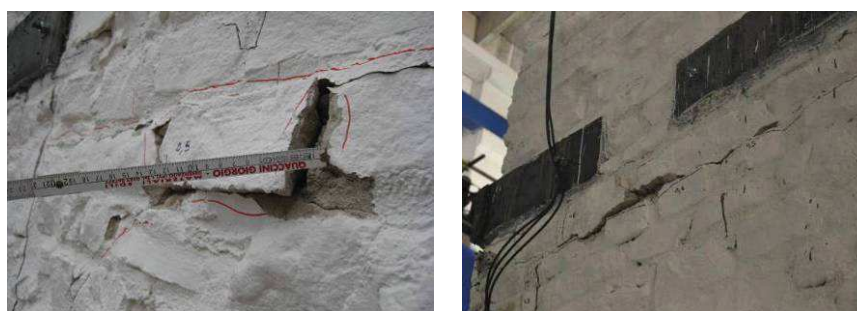
Figure 14. Decohesion of masonry blocks after the test with nominal PGA of 0.30g (aftershock): spandrel in the West façade (left), top of the base pier of the East wall (right).
