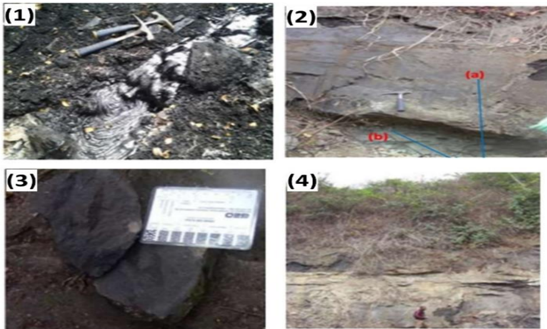
Fig. 3: Hydrocarbon indices in the study area (Mavuma block): (1) Bitumen seepage; (2) A non-impregnated original rock (a), overlying the impregnated part (b); (3) Sample of sandstone impregnated with hydrocarbons; (4) Limestone horizon in a sandstone formation impregnated with hydrocarbons
