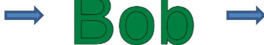
After applying Break Apart : child shapes fill with color, rather than being “holes” inside the letters
