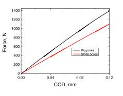
F-COD curve matching the instance of crack entering the cut-out of microstructure
