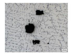
Both tomographical and metallographical surface characterization testifies to the existence of small pores (diameter around 20 mm) and big pores (200-400 mm).
