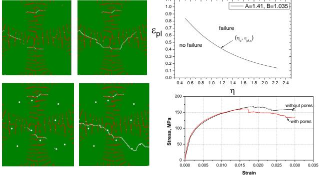
Porosity effects the crack propagation in microstructure deviating the crack from its initial path at the later stages of simulations and the stress-drop on stress-strain curve is clearly pronounced in the microstructure with porosity.
