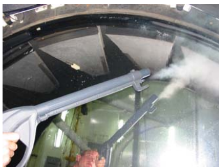
Vapour cleaning (left) and drying (right) INT primary mirror.
