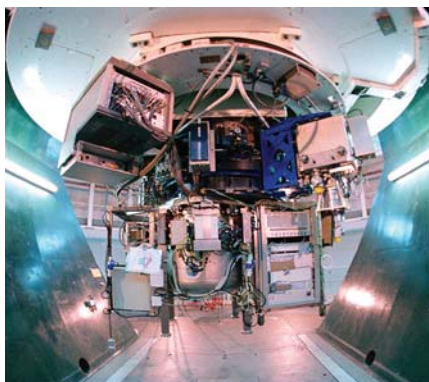
Figure 1 (top left). LIRIS mounted on the WHT Cassegrain focus. LIRIS cryostat can be seen at the bottom of the telescope focus, with the two electronics racks at both sides. Figure 2 (top right). The globular cluster M5 in the J band. The FWHM of the PSF was 2 pixels corresponding to 0.5". The image quality is very good over the whole field of view (4.2 arcmin 2 ). Figure 3 (right). Arrival of LIRIS at the WHT in January.
