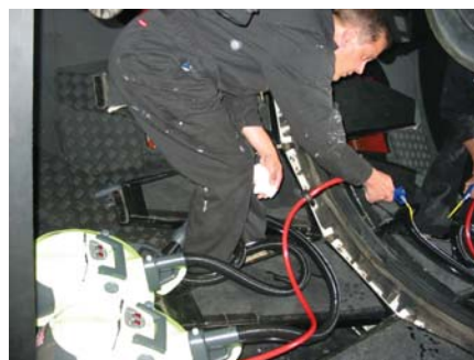
Vapour cleaning (left) and drying (right) INT primary mirror.
