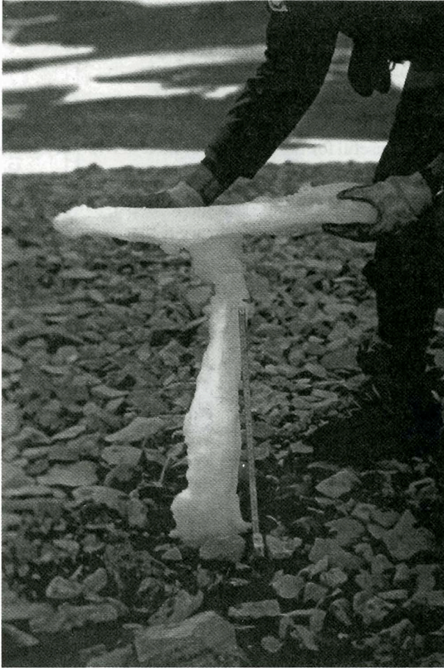
Figure 2.37. Photograph of a large ice column, capped by an ice layer that had been removed from a cold snow cover in the Arctic (Phil Marsh, NHRI). The column was formed by meltwater refreezing where ponded along a horizontal structural divide in the snowpack and in a vertical preferential flow path.
