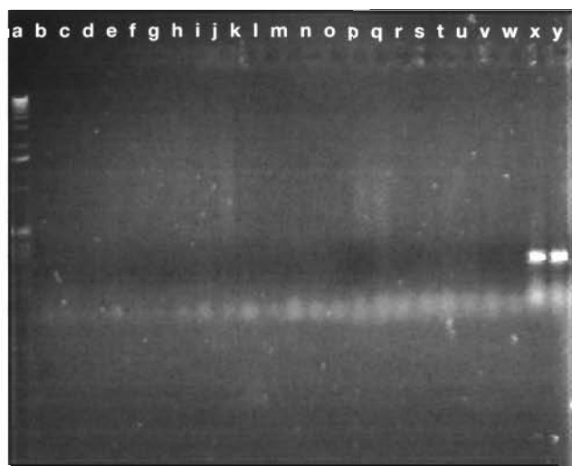
Fig. 5. Photograph of a 1.8% agarose electrophoresis gel showing the PCR amplification reaction products using various genomic DNA samples. Lane a: molecular weight markers (MWM) (BRL 1 kb ladder); Lane b: Staphylococcus aureus ; Lane c: Staphylococcus spp.; Lane d: Aeromonas spp.; Lane e: Streptococcus agalactiae ; Lane f: Corynebacterium bovis ; Lane g: Serratia marcescens ; Lane h: Enterobacter cloacae ; Lane i: Klebsiella pneumoniae ; Lane j: Pseudomonas spp.; Lane k: Vibrio spp.; Lane l: Yersinia enterocolitica ; Lane m: Mycoplasma bovirhinis ; Lane n: Mycoplasma Group 7; Lane o: Mycoplasma ovipneumoniae ; Lane p: Mycoplasma arginini ; Lane q: Mycoplasma dispar ; Lane r: Mycoplasma agalactiae ; Lane s: Mycoplasma bovirhinis ; Lane t: Mycoplasma bovirhinis ; Lane u: Mycoplasma bovis (type strain); Lane v: MP2 ; Lane w: no template; Lane x: isolated Mycoplasma ( MP1 ); Lane y: recombinant pUC19 (positive control)
