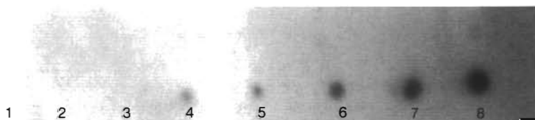
Fig. 3. Sensitivity of the DNA probe MP1/1-2 in the dot-blot procedure. Dilutions of a preparation of Mycoplasma ( MP1 ) with a known titre were added to a crude homogenised healthy prawn sample No. 2 (see Fig. 2), and then extracted DNA from the experimentally seeded samples was subjected to the dot-blot procedure. Samples contained (1) 10^1 , (2) 10^2 , (3) 5 \times 10^2 , (4) 10^3 , (5) 10^4 , (6) 10^5 , (7) 10^6 , (8) 10^7 CFU \text{ml}^{-1} of prawn isolated Mycoplasma
