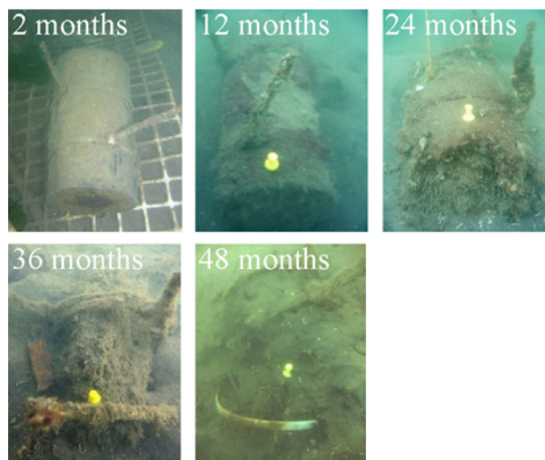
Fig. S3 State of fragmentation of some of the cedar logs after 2, 12, 24, 36 and 48 months.
