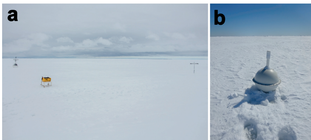
Fig. 3.1.2.2.2: (a) PS96/H009: Autonomous Weather Station (left), Ice Mass Balance buoy (middle), and snow depth buoy (right). (b) PS96/H001-BUOY-SVP-1: SVP buoy.
