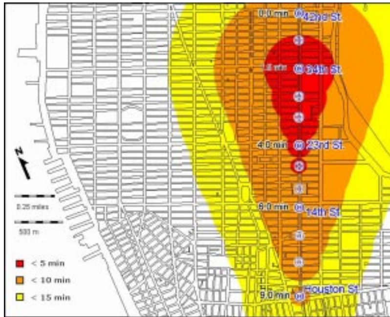
Map 3.5-1: East Side LRT Line Accessibility up to 2 miles Journey times from 42 nd Street traveling south
