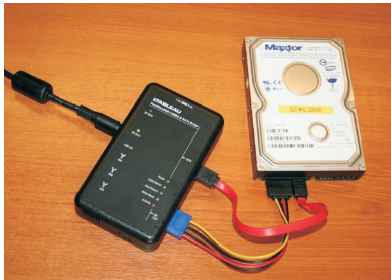
FIGURE 4. An image is "an exact bit-stream copy of all electronic data on a device, performed in a manner that ensures that the information is not altered." (Source: NIST glossary.) This portable write blocker is attached to and copying a hard drive for forensic purposes. (Source: Wikipedia.)
