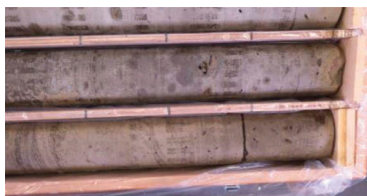
Figure 63. Successful grouting shown by solidified soil cores.
