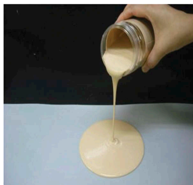
Figure 76. Super heavy mud water for radioactive shielding (study at Waseda University).
