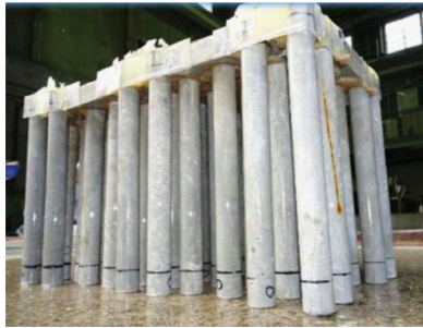
Figure 44. Excavated shape of columns with head connection (full-scale model, after Dr. Naoki Takahashi).
