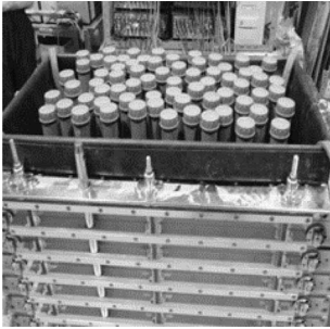
Figure 36. 1-G shaking model of liquefaction-prone ground with vertical columns for restriction of cyclic shear strain.
