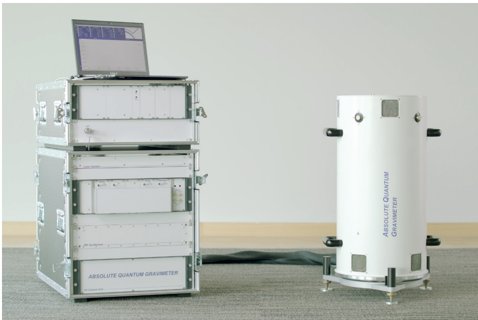
Picture of the Absolute Quantum Gravimeter. The instrument is composed of the sensor head (right side of the image) where the gravity measurement is performed, and the control unit (left side of the image)
