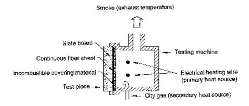
Figure 1 Overview of testing machine
