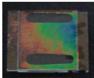
Fig 1. Reflection changes with temperature in a mixture of calamitic liquid crystals and chiral dopant (left). All the colors are visible at once when the cooling cell experiences a temperature gradient (right).
