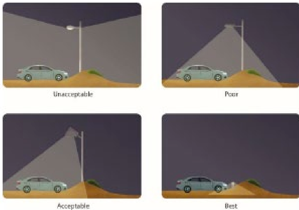
Figure 46: Lighting options for a parking lot. Reproduced from source: Pendoley et al. (2020) adapted from Withering and Martin (2003)
