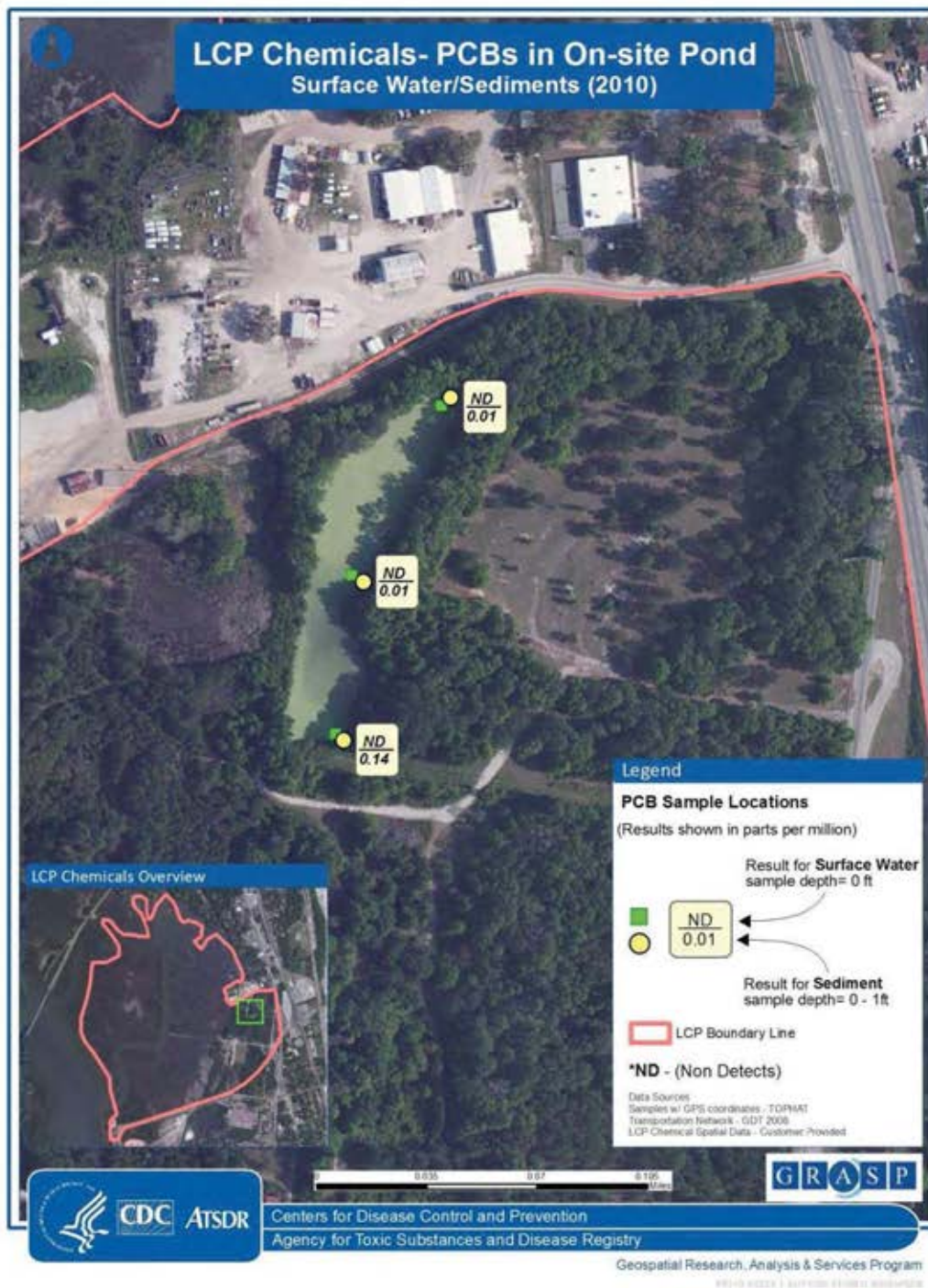
Figure 18. Sampling Locations Showing Concentration of PCBs in Surface Water and Sediment in On-site Pond, 2010
