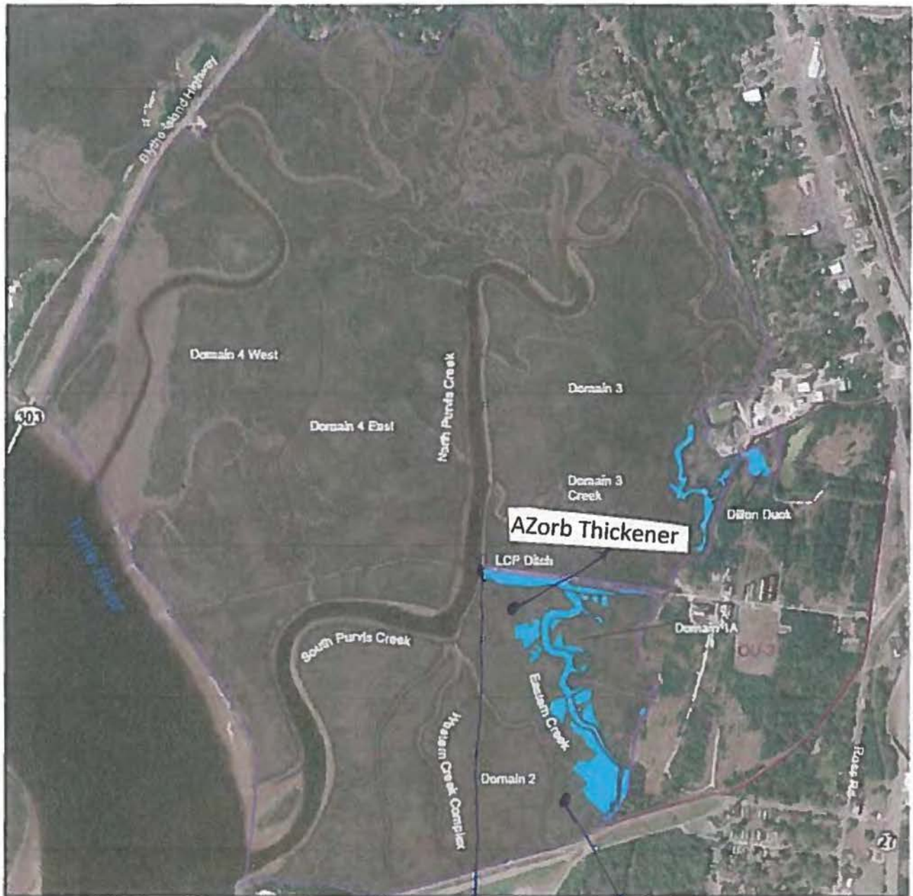
Figure 9 – Sediment Remedy Alternative 4: Sediment Removal – 18 Acres
