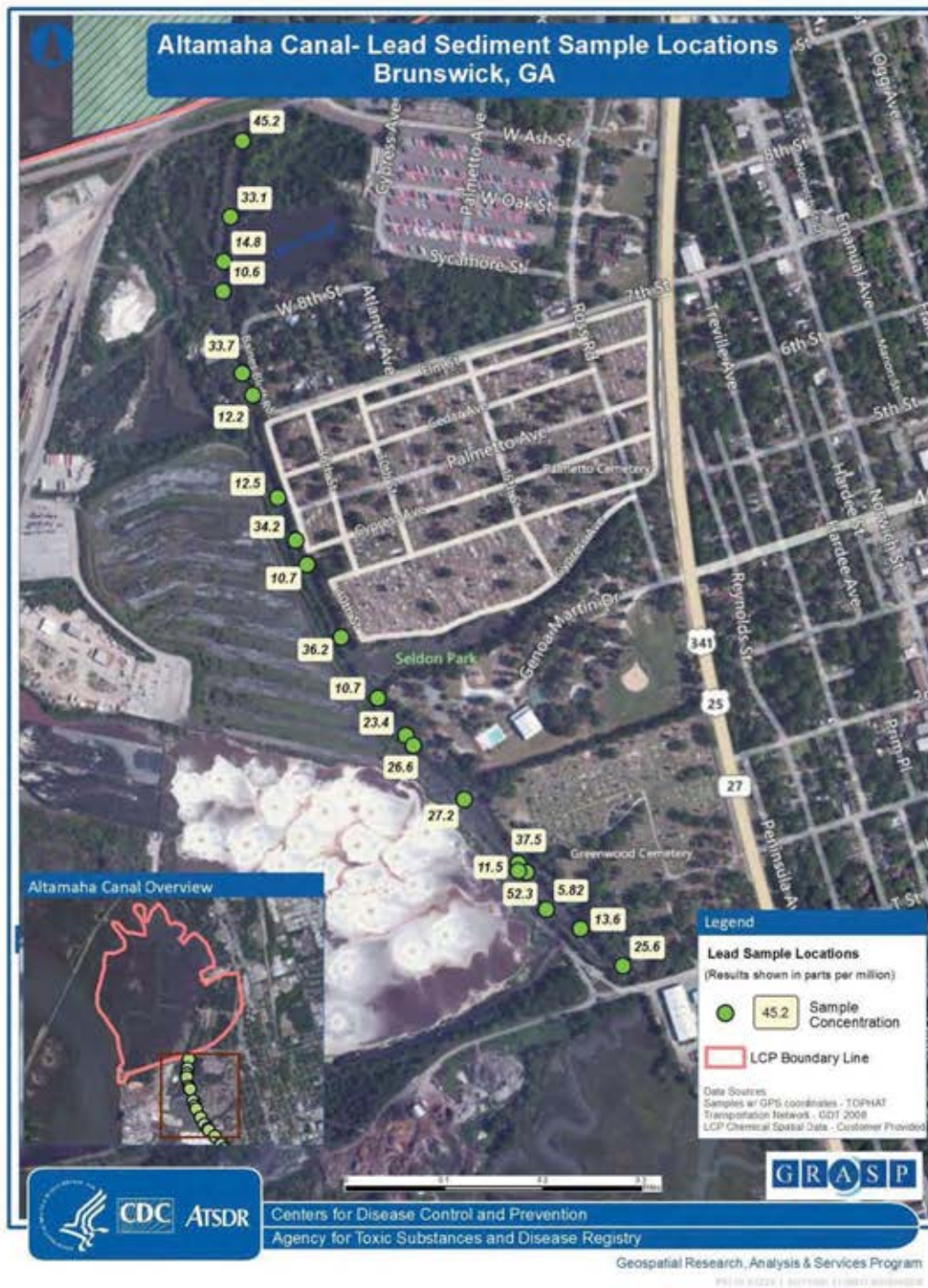
Figure 29. Sampling Locations Showing Concentration of Lead in Sediment in Altamaha Canal, 2011 Just South of the LCP Chemicals Site.
