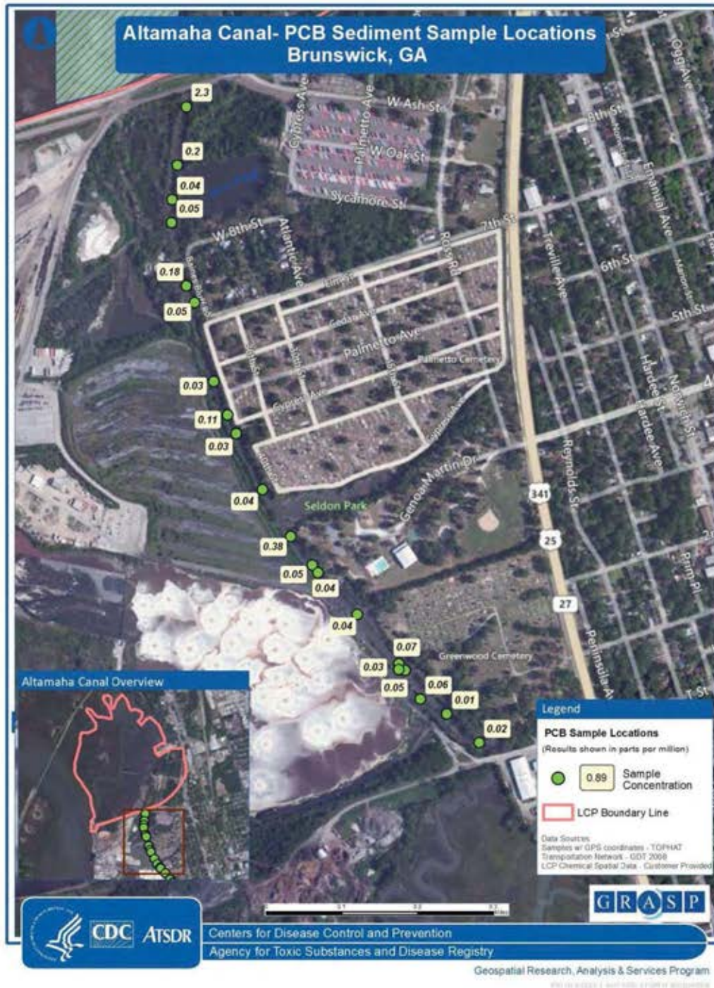
Figure 26. Sampling Locations Showing Concentration of PCBs in Sediment in Altamaha Canal, 2011 Just South of the LCP Chemicals Site.
