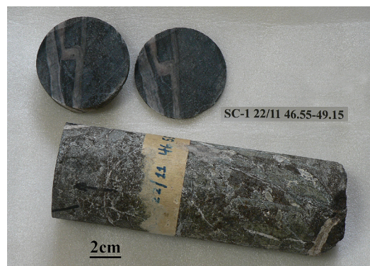
Fig. 9. Drilling core at 46.6m in depth, “Phoscorite.” Mine of Goiasfertil S.A., Catalão (GO).
