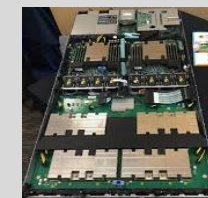
1U-4G Dell PowerEdge C4130
