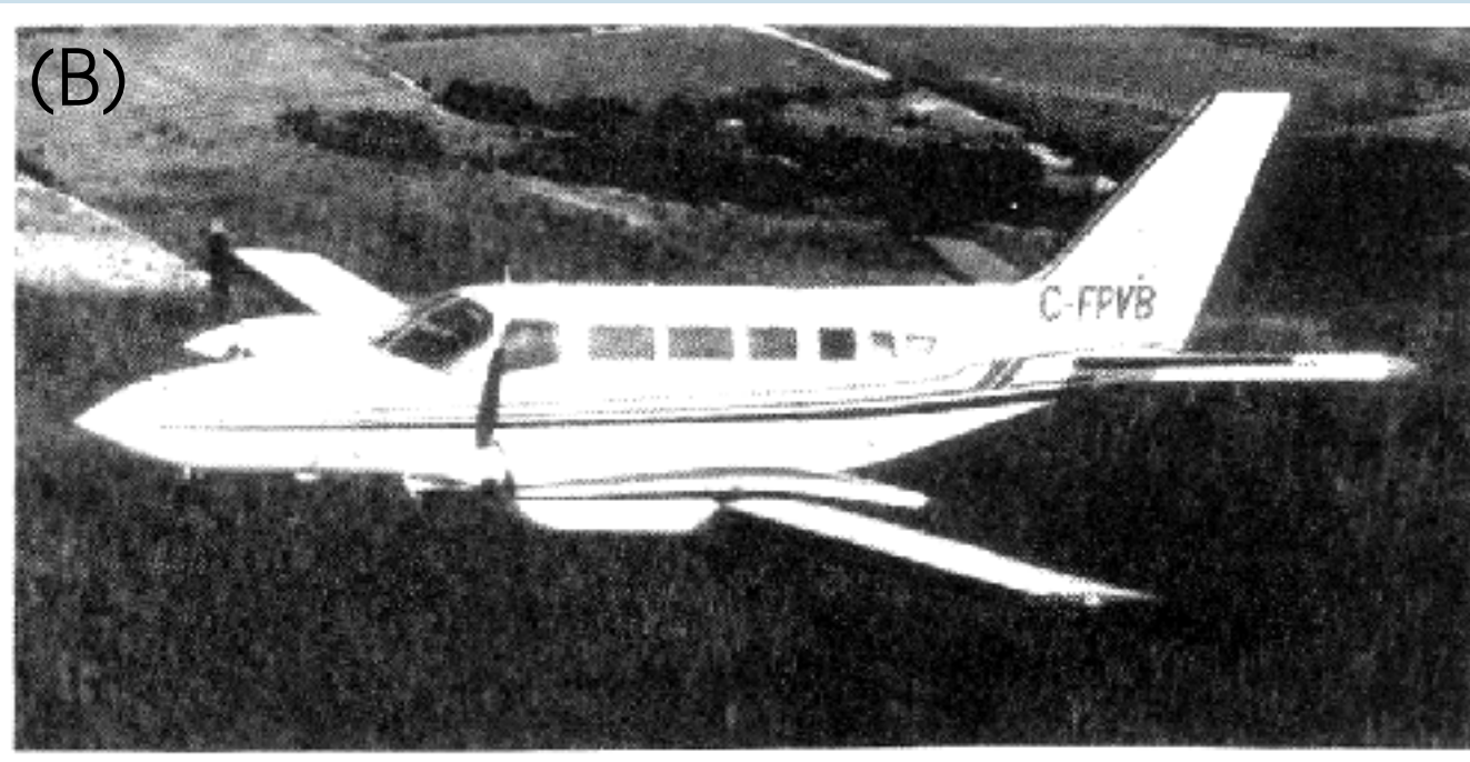
Fig. 12: (A) Eurocopter AS350B towing three instrument pods. They are from the top 2-channel VLF-EM, total-field cesium magnetometer, and a 5-frequency electromagnetic induction system. (B) Cessna 404 fixed wing aircraft with a total field magnetometer mounted in a tail stinger. 1
