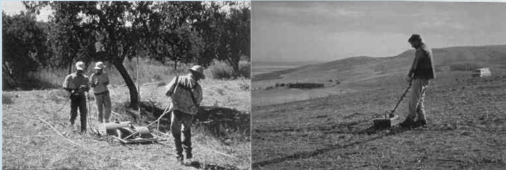
Fig. 52: Measurements with Ground Penetrating Radar. Left: 120 MHz antenna system (bistatic). Right: 500 MHz antenna system (monostatic). 7
