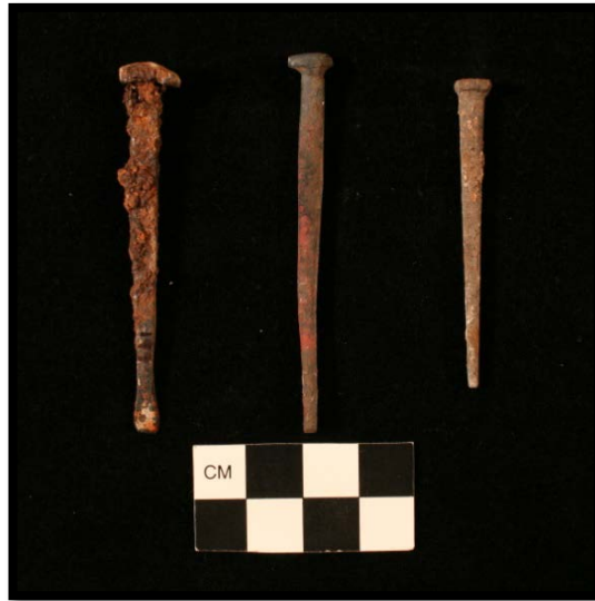
Figure 13. Nails: Left, Hand Wrought; Center, Early Machine-Cut; Right, Late Machine-Cut.
