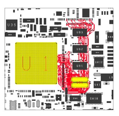
The best time to simulate a PCB for signal integrity is after layout and before fabrication. Taking the time to simulate becomes more important as speeds increase. There are now more factors that can lead to signal integrity problems. Common problems that can arise include reflections at the interconnects (mismatched impedances), electromagnetic coupling between the traces, and grounding issues. If not addressed, these problems can lead to signal distortion and attenuation.
