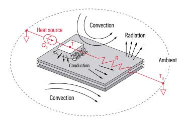
with temperature. This makes it difficult to estimate the final temperature of a via with hand calculations. Instead, simulation analyses that take into account all the thermal effects are necessary to determine the final via temperature.
