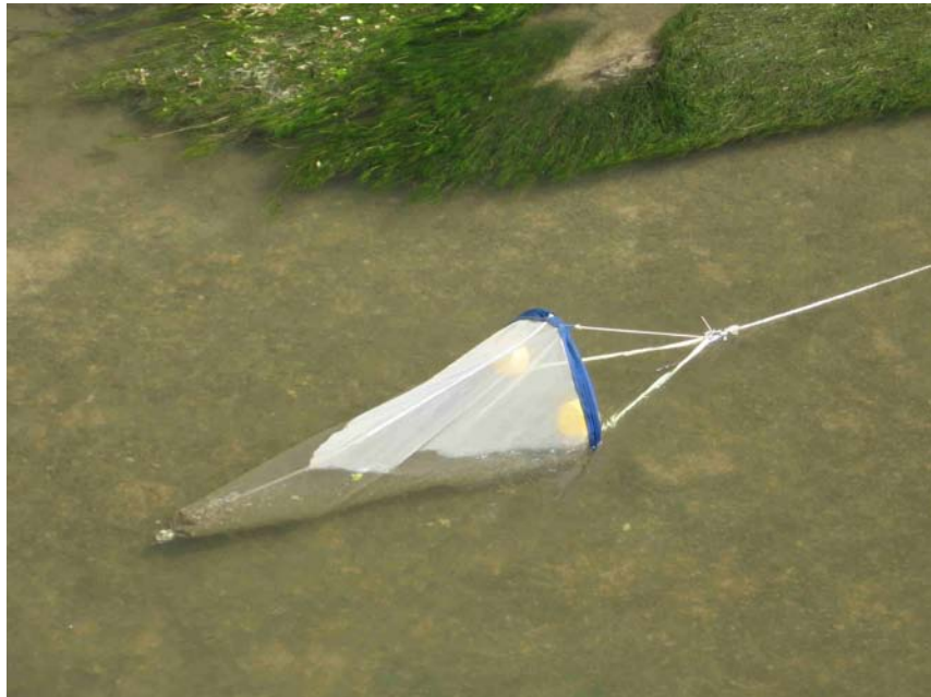
Photo 5. Driftnet used to collect exuviae (diameter opening 60 cm)
