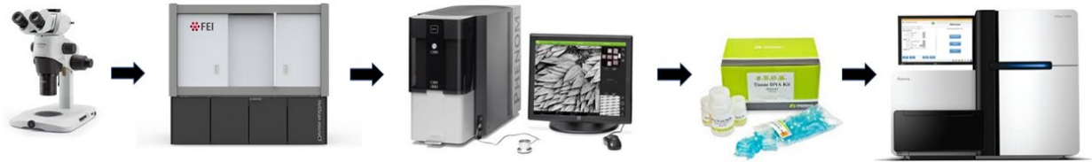
Figure 4. Proposed data collection workflow. Specimens are imaged using stereo light microscopy with extended focal imaging. Specimens are then contrasted and imaged using micro-CT scanning. Subsequently, specimens are dried and imaged using low acceleration voltage SEM. DNA is then extracted (sclerites are retrieved and mounted on a slide as a permanent voucher) for barcoding or sequencing library preparation.
