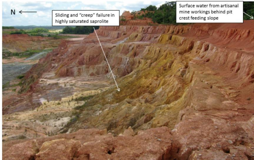
Figure 4 – Example of a creep style failure in highly saturated saprolites along the south wall of Royal Hill, south pit
