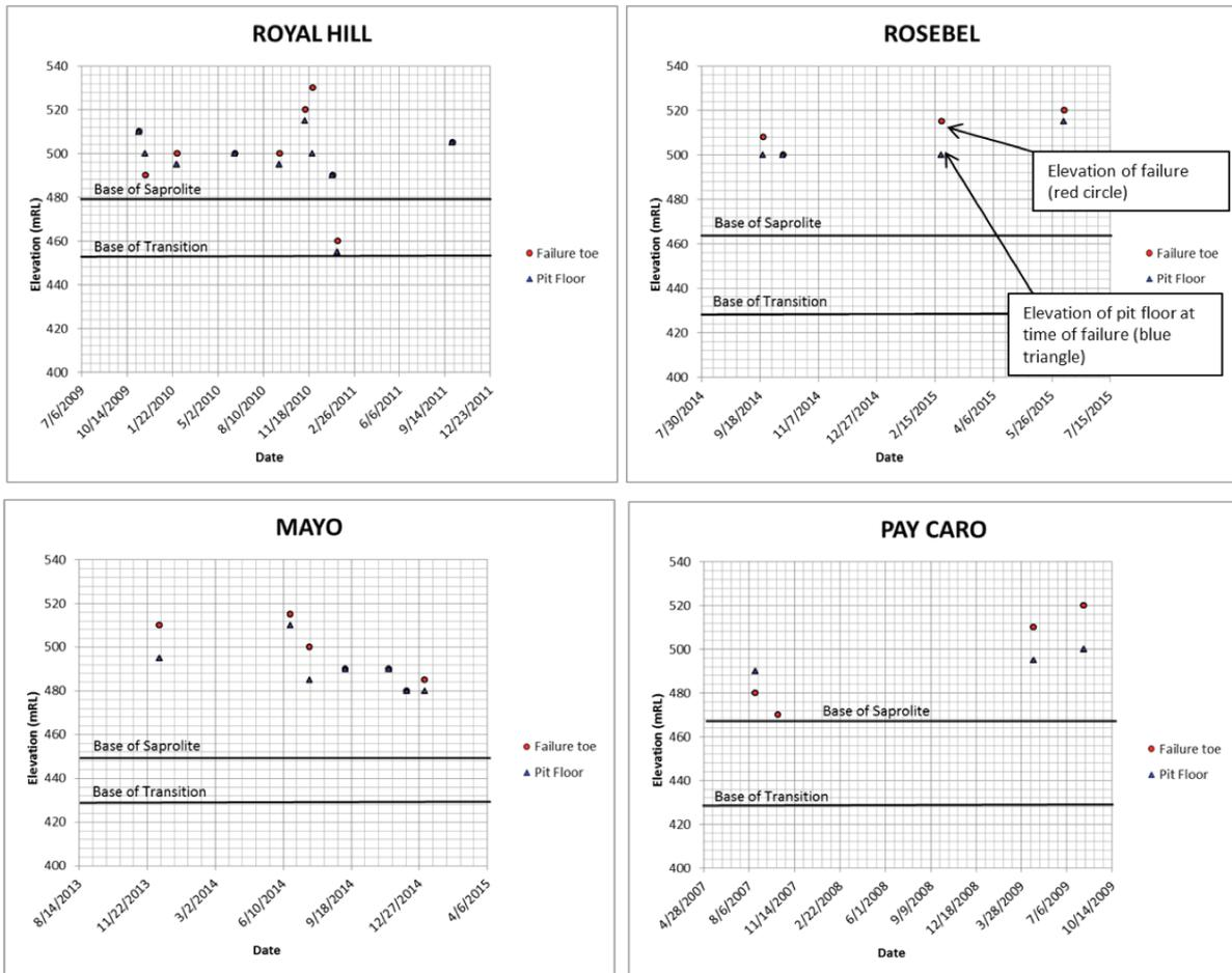
Figure 10 – Plots of saprolite failures (red circles) and elevations of the pit floor at time of failure (blue triangles) relative to the weathering surfaces. The majority of slope failures are seen to occur while the pit floor is still in saprolite
