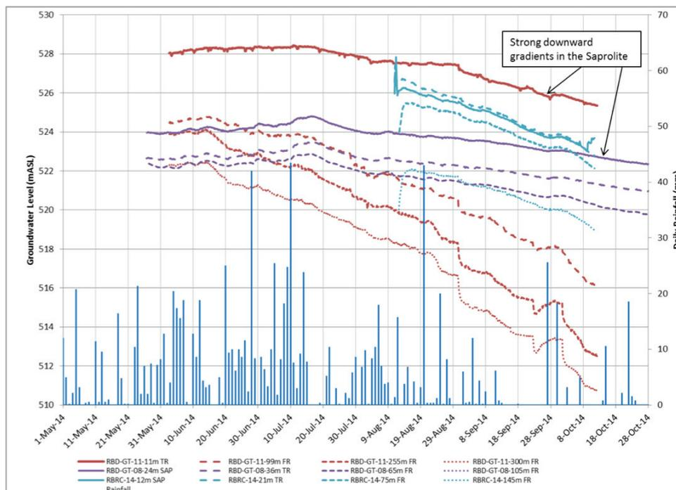
Figure 8 – VWP data from the north wall of Rosebel Pit showing strong downward gradients in the saprolite and transition as mining progresses
