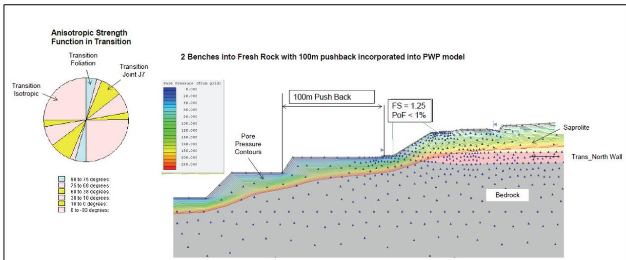
**Figure 12 – Example of stability model showing the anisotropic strength function applied to transition material and contours of pore pressure grid for a 100 m push-back**
