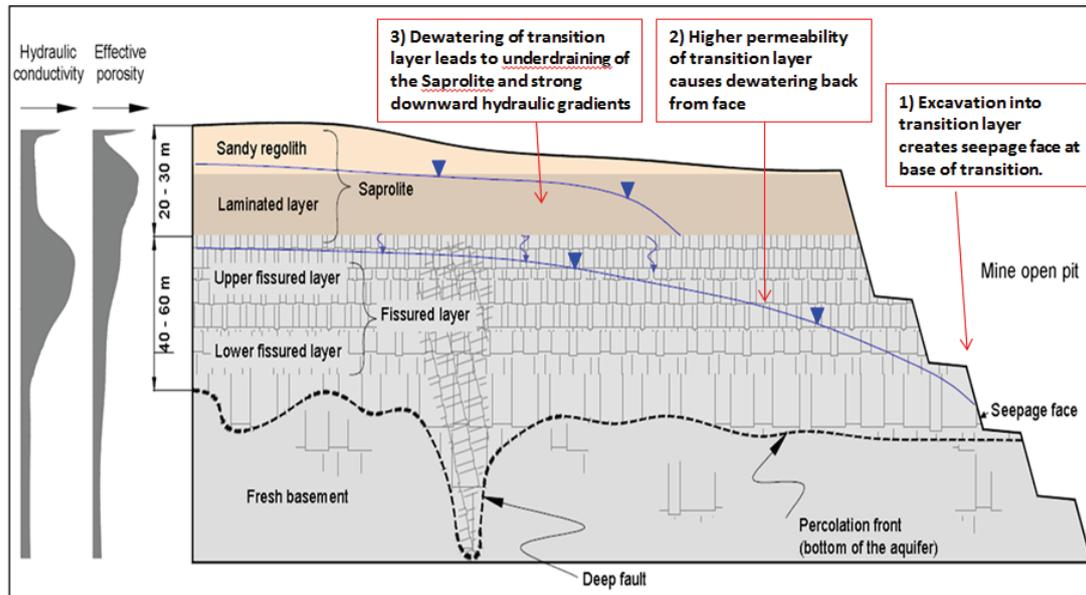
Figure 7 – A conceptualization of groundwater flow for an open pit mine located in a deeply weathered tropical environment. Based on work by Wyns, Baltassat, and Lachassange, 2004; Dewandel, 2006; Elster, Holman, Parker, and Rudge, 2014; and SRK
