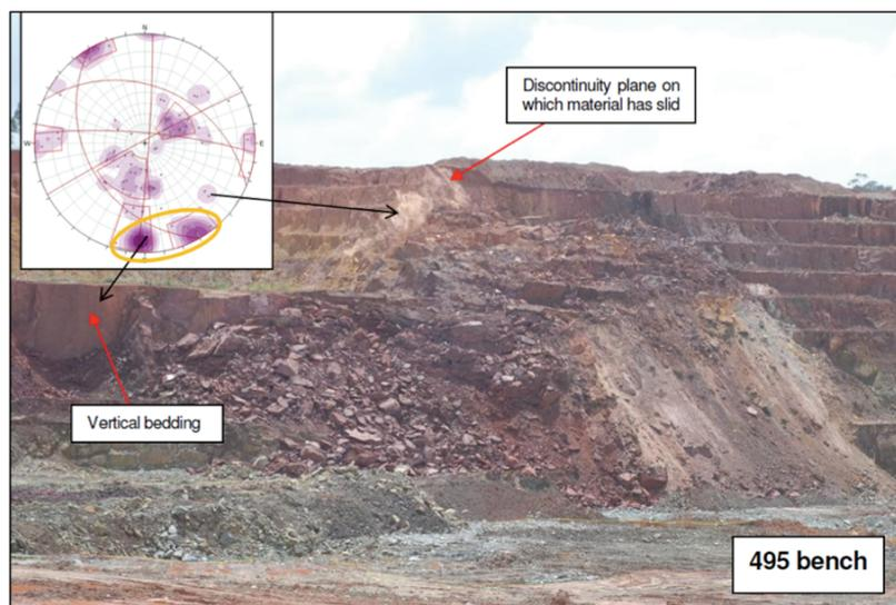
Figure 5 – Complex, toppling-style failure impacted by relict structures in the saprolite and transition
