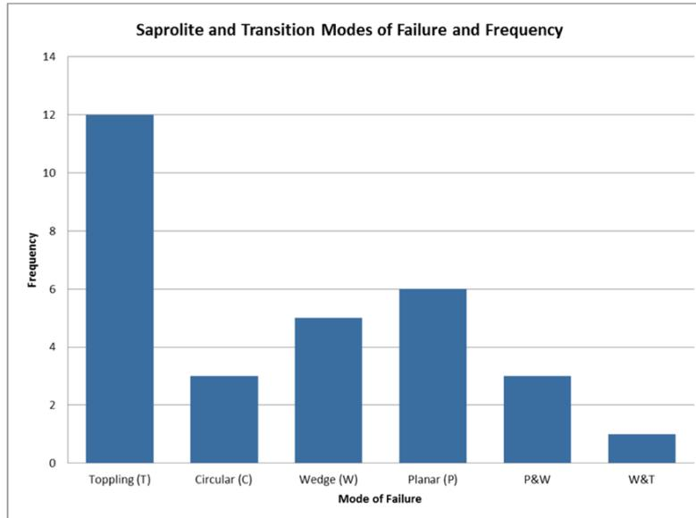
Figure 6 – Graph showing the number of failures observed to date and the primary failure mode. The numerous toppling and planar failures indicate the impact of relict structures on slope stability
