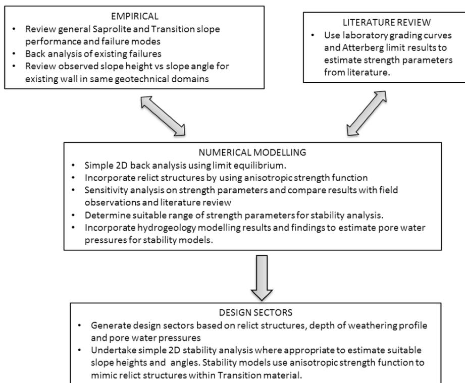
Figure 2 – Saprolite slope design methodology
