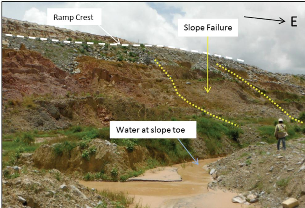
Figure 11 – Slope instability in saturated saprolite slopes on the northern wall of Mayo Pit
