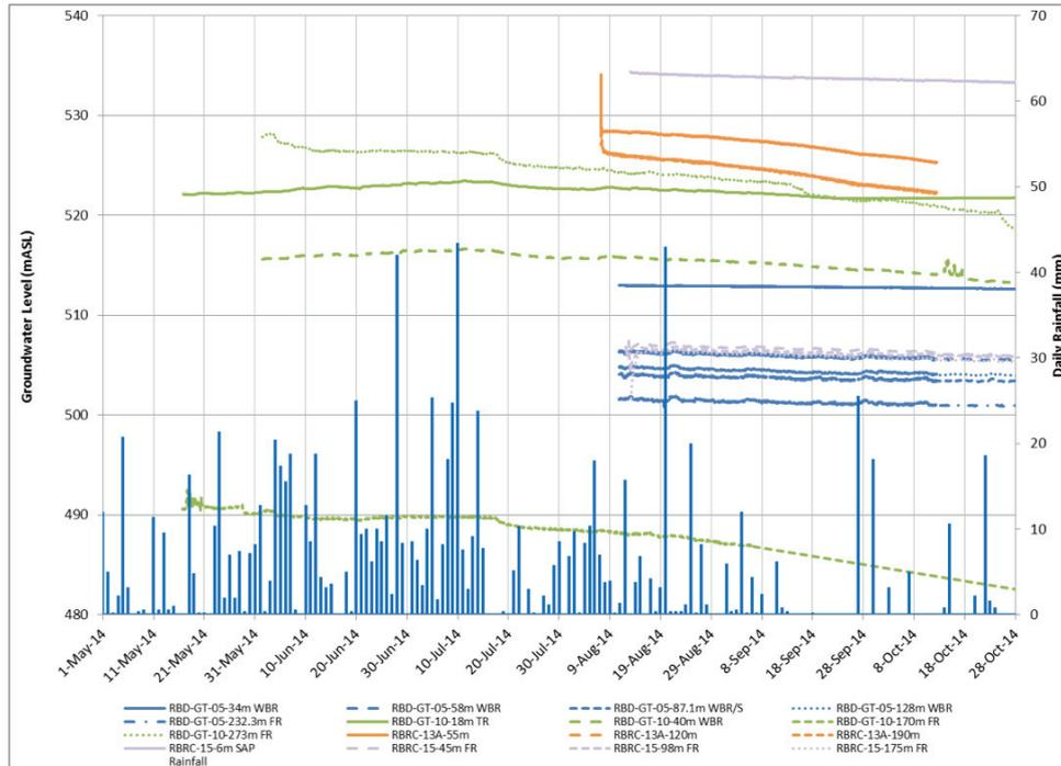
Figure 9 – VWP data from the south wall of Rosebel Pit showing relatively little response to mining in some areas. This is thought to be due to a structure striking immediately behind and parallel to the pit wall
