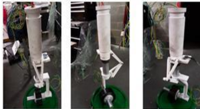
Figure 18: Completed assembly of 3D printed BTR v. 1 Oleo strut with sensors attached
