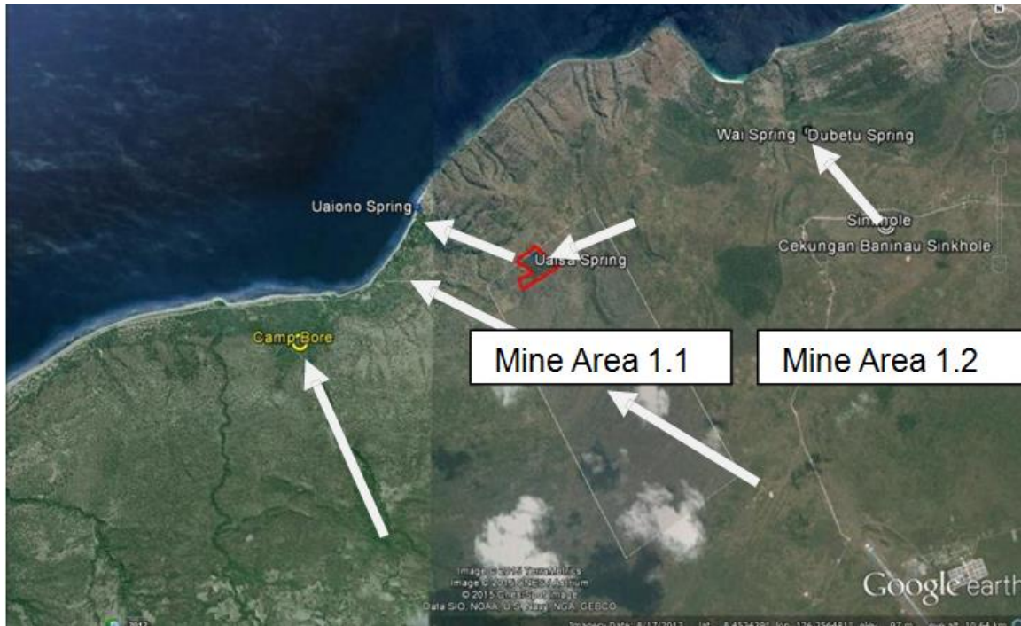
Figure 27 Inferred Groundwater Flow Paths
