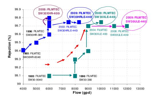
Figure 2: Evolution of spiral wound module performance, illustrated by example of the DOW<sup>TM</sup> FILMTEC<sup>TM</sup> seawater desalination product range
