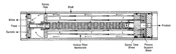
Figure 1: Hollow fine fiber module and process [DuPont, 1983]
