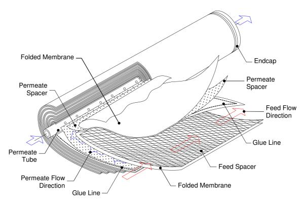
Figure 3: Configuration of spiral wound membrane module for reverse osmosis.
