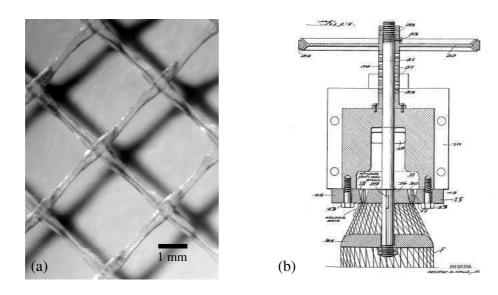
Figure 4: (a) Biplanar extruded netting is comprised of two intersecting sets of parallel, extruded strands. (b) An early patent was obtained by Nalle (1962).
